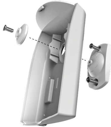
FIG 2. Installation of the Standard Swivel Bracket.
