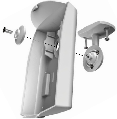
FIG 3. Installation of the optional Deluxe Swivel Bracket.
